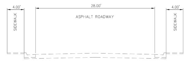
Figure 5: Existing Typical Section Parsifal Street Looking North
